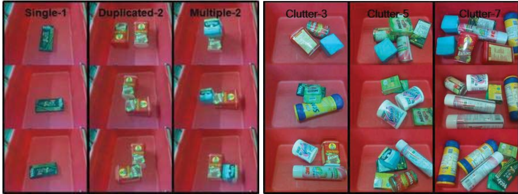
(a) Scenes are designed with single, 2 duplicated, or 2 different objects, adjacent or occluded with each other. All brandnames are facing up. (b) Scenes are arranged with 3, 5, or 7 objects in clutter. The brandnames are either facing upward or downward, and may be occluded.
