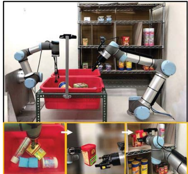
Fig. 1: We use the product brandname, one of the “semantic labels,” for pose-aware placement of objects. We perform active manipulation using two cooperative robotic arms to handle object occlusions (e.g., brandname facing downward). Bottom left to right: A vacuum gripper picks a target object using object-level or brandname-level affordance prediction, the brandname is then used to predict grasp, and finally a two-finger gripper places the target object on the shelf.
