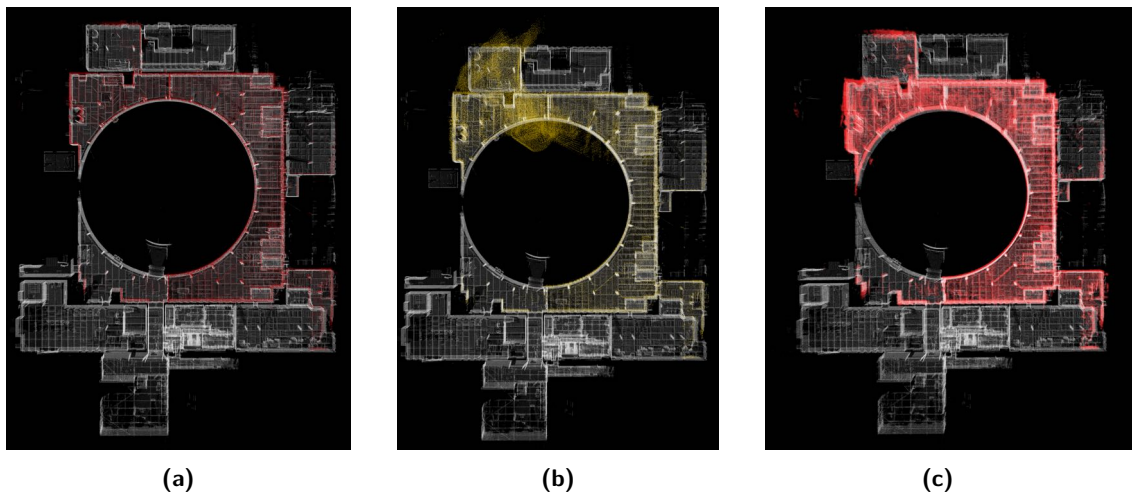
Figure 17. Comparison of ground truth map (white) and maps generated using the LeGO-LOAM algorithm (colored): (a) Before rapid jump; (b) After rapid jump; (c) Map recovery based on confidence tests and corresponding recovery procedure.
