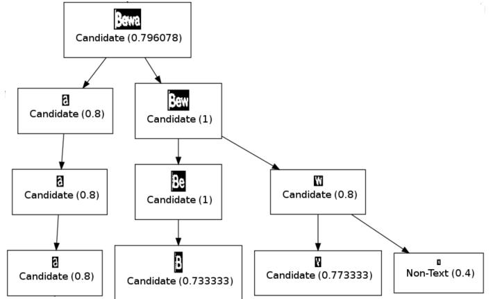
Fig. 3. MSER component tree. Each node was classified as (potential) text, or as non-text, based on shape descriptors including compactness, eccentricity, and the number of outer boundary inflection points.
