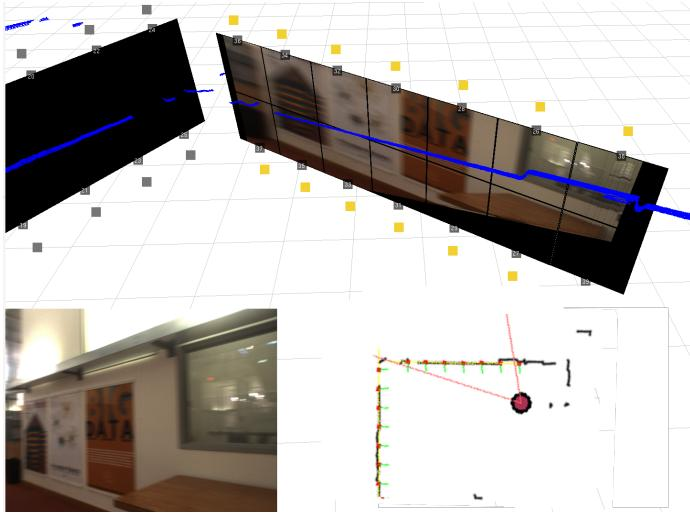
Fig. 2. Top: Visualization of a 3D environment. Each yellow or black label represents an  $1 \times 1$  meter tile. The yellow ones are in camera field of view, and the black ones are discovered by LIDAR, but not by camera. Bottom left: A camera frame. Bottom right: Map generated by the SLAM module (black lines) with generated tiles overlaid (origins in red; normals in green).
